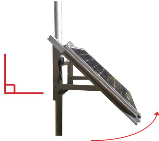
5. Un-tighten the 6 bolts on the inside of the frame that are used to hold the solar panel at a right angle. Do NOT completely removed the bolts.
