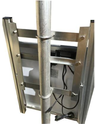
4. Loosen the 6 bolts on the inside of the frame. DO NOT completely remove these bolts. Lift the bottom of the solar panel until the attached arms holding it are angled at 90 degrees. Tighten all 6 bolts again and face the panel north.
