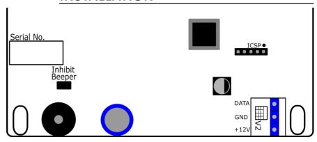
Connect +12V, GND and DATA to an Energizer or Monitor.
