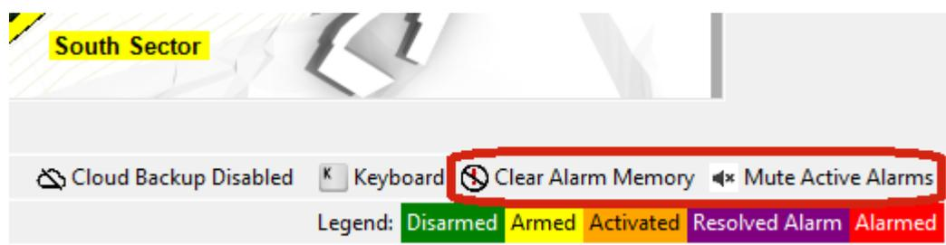
Figure 9 - The “Clear Alarm Memory” and “Mute Active Alarms” button
