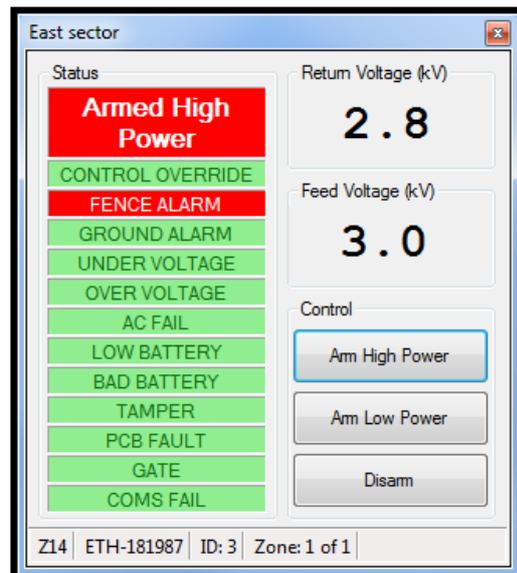
Figure 7 - Extended zone information showing an alarm
