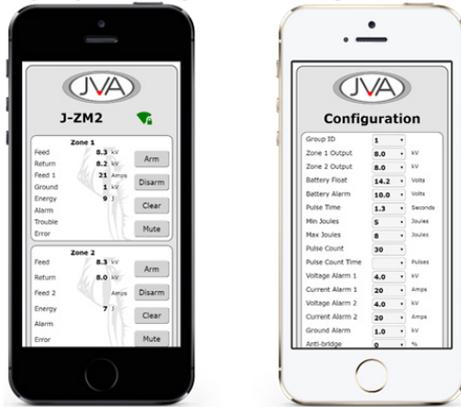
Figure 4 - Virtual Keypad Interface
