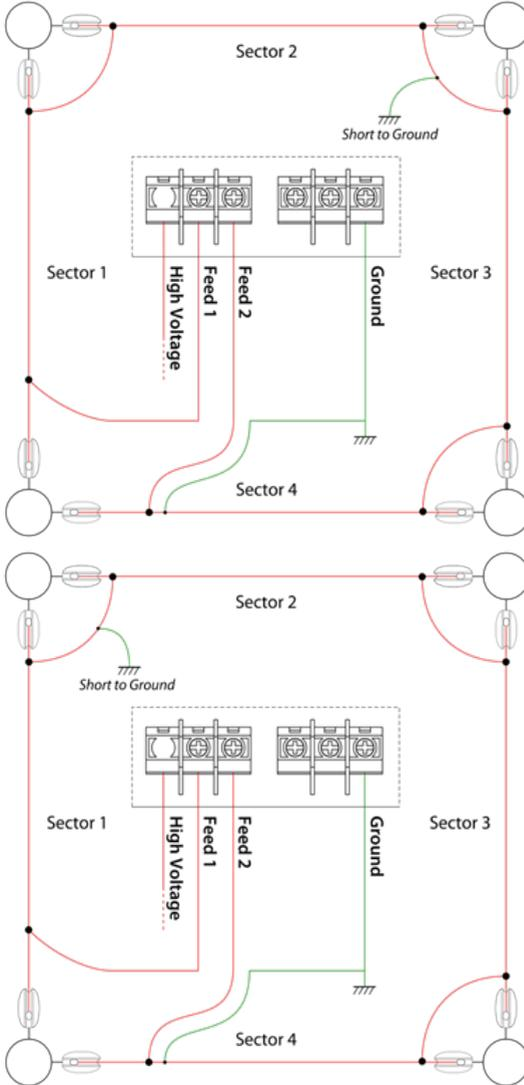
Remove the short at the end of Sector 1 and move it to the end of Sector 2. When the energizer goes into alarm it will display Sector 2 – Short.
