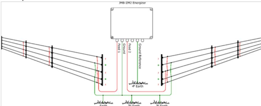
Figure 2 - Typical JMBx-ZM2 setup
