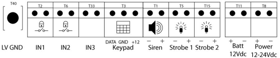
If no battery is connected, the combined power for all 3 outputs can only be less than 0.5A.
