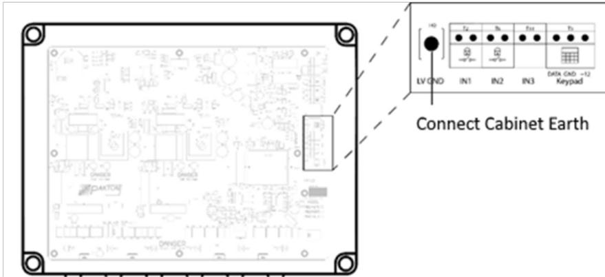
Note: **Do not** connect LV GND to the fence earth rod. It may be connected to a cabinet earth
