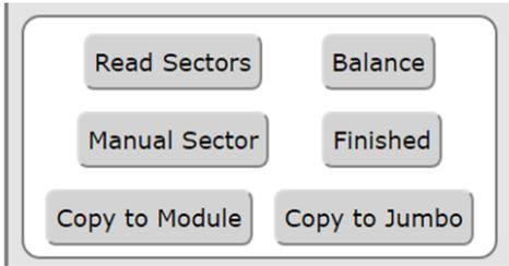
To save the sector details to the Virtual Keypad, select the “Copy to Module” button from within the Sectorize options page. This allows the Virtual Keypad to hold the information of the sectors that have been set from the energizer. Note that this data is stored in the Wi-Fi module (pluggable) on the PCB, not on the phone you are using to view it.
