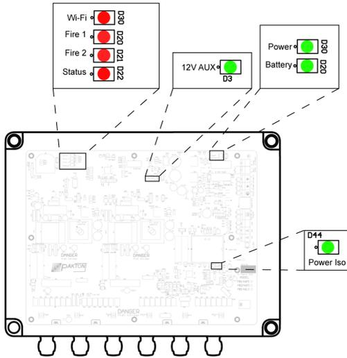
The status LED's on the PCB of the JVA JMB series energizers allow the user to quickly check the status of the unit and if any action needs to be taken.
