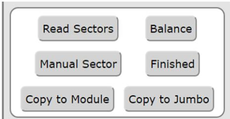
To load the sector settings from the Virtual Keypad onto the energizer, select the “Copy to Jumbo” button from within the Sectorize options page. This allows previously configured sector options to transfer from a previously configured energizer to the current one.
