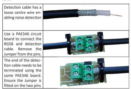
The wires connecting to the PAE346 board should be secured using cable ties before being enclosed in a weather proof junction box (MHC017) to protect it from the weather and insects.
