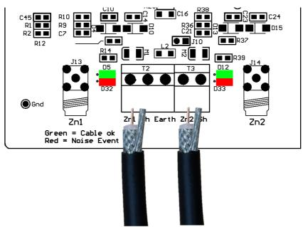
NOTE: The earth terminal must be connected to stop 50/60Hz noise from affecting the system
