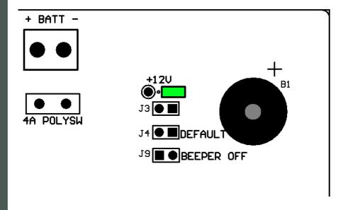
Jumpers located on the top right hand side of the board
