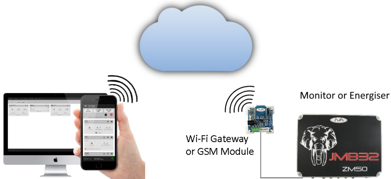
Password protected control via the Cloud Router Web App (Mobile friendly)
