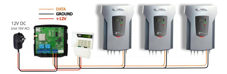
Confirm the KPB is flashing, the ERROR light is not flashing, and the GSM light is fully lit. Clip on the case front. If the GSM light is on, your JVA Cellular Gateway is ready to use.
