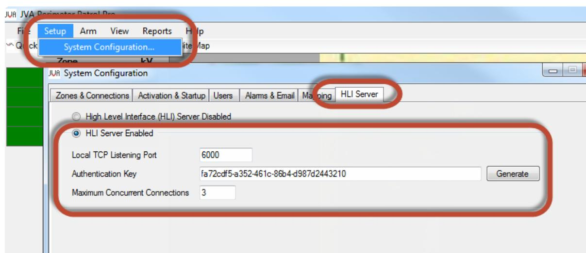
Figure 1 - Enabling HLI Server to accept HLI connections
