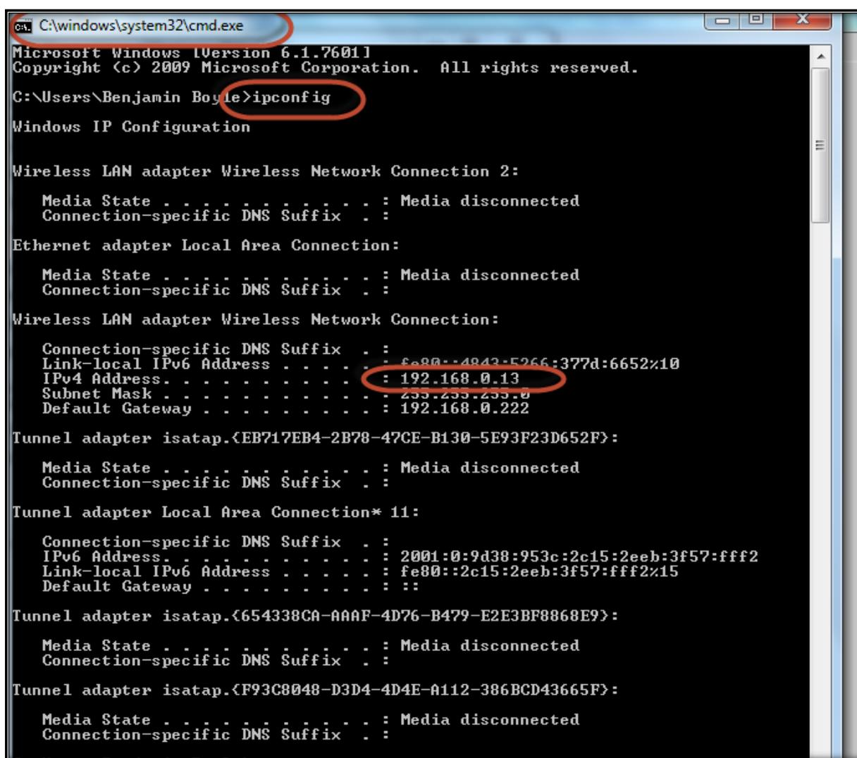
Figure 2 - Finding out the computer's static IP Address
