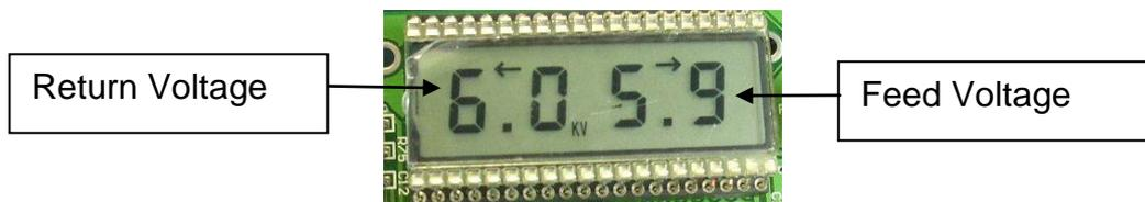
8. Calculate the return calibration factor = (Actual Voltage / Displayed voltage \*100) – 100
